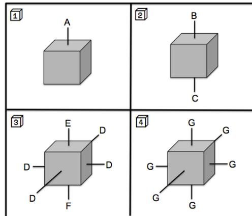
Cubes can be glued together by combining them in solution with linker DNA. Linker DNA contains two "sticky ends" that are complementary to other sequences. For example, a linker containing sequence A'-C' will stick to cube face A. To glue face A to face C, we would add linker A'-C' to a solution containing cubes patched with sequence A and cubes patched with sequence C:
